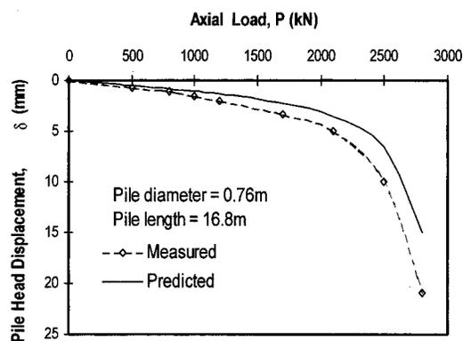
**Fig. 12.** Predicted and measured load-displacement curve for Piedmont pile
