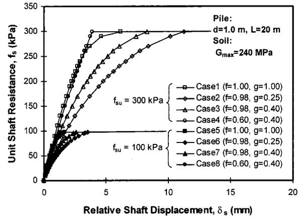
Fig. 6. Effect of factors  $f$  and  $g$  and ultimate skin friction of  $t$ - $z$  curves
