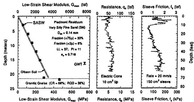
**Fig. 11.** Profiles of  $G_{max}$ ,  $q_c$ , and  $f_s$  at Piedmont test pile site (after Mayne 1995)
