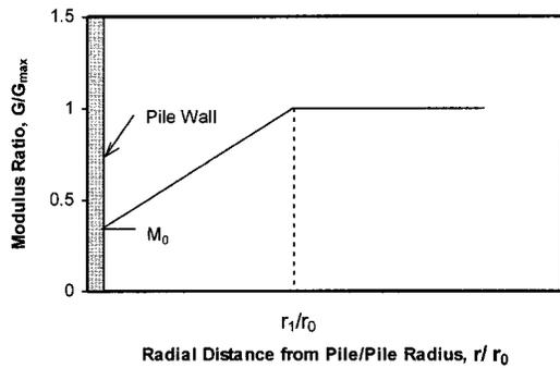
**Fig. 4.** Idealized radial distribution of soil modulus ratio (after Kraft et al. 1981)
