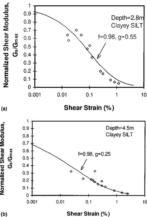
**Fig. 16.** Deduced  $G_s/G_{max}$ -shear strain data and best fitting curve for Singapore pile
