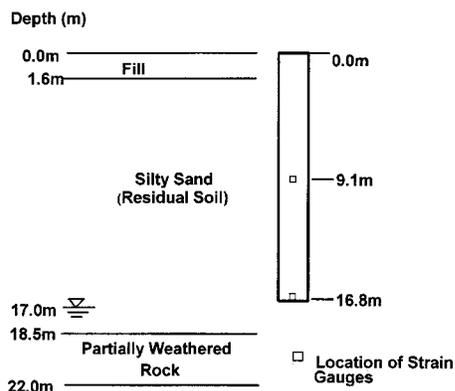
**Fig. 10.** Soil profile at Piedmont pile location and pile instrumentation
