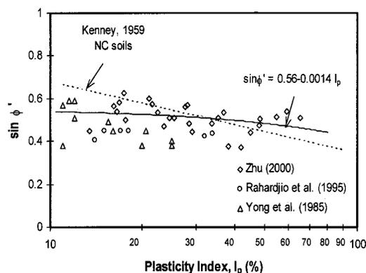
**Fig. 8.** Relationship between  $\sin \phi'$  and plasticity index for residual soil of Jurong Formation
