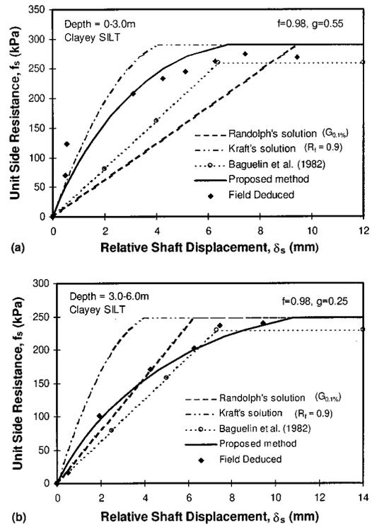
**Fig. 17.** Comparison of predicted and field deduced  $t-z$  curves for Singapore pile
