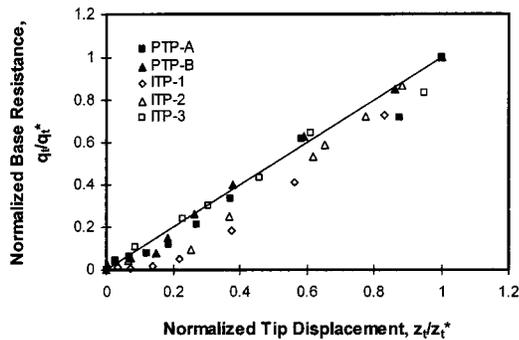
**Fig. 9.** Normalized load-transfer curve for pile tip
