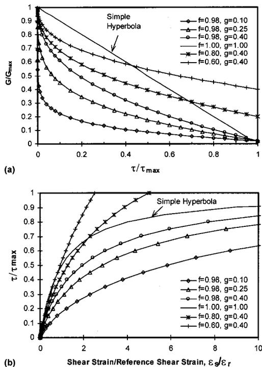
Fig. 2. Effect of stress or strain level on shear modulus: (a) theoretical modulus degradation curves; (b) theoretical stress-strain curves
