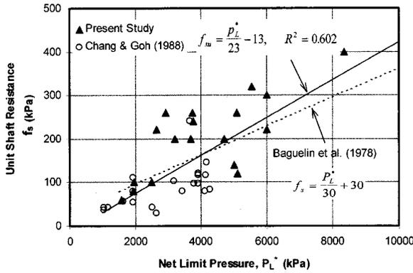
Fig. 5. Relationship between  $f_{su}$  and  $p_L^*$  for residual soils of Singapore (after Zhu 2000)
