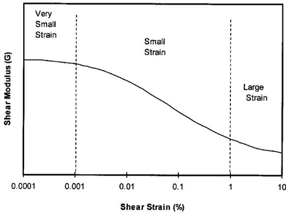
Fig. 1. Characteristic ranges of stiffness of soils
