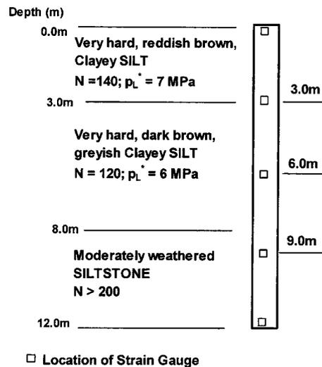
**Fig. 14.** Soil profile at Singapore test pile site and pile instrumentation
