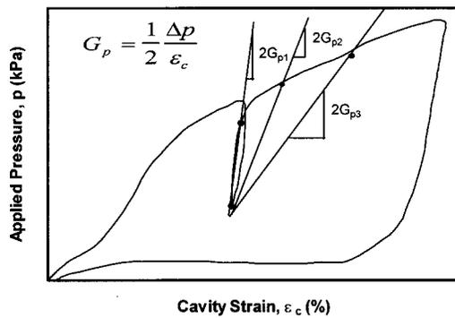
Fig. 7. Deduction of modulus from pressuremeter expansion curve
