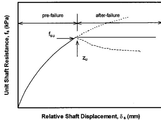
Fig. 3. Schematic presentation of proposed  $t$ - $z$  curve
