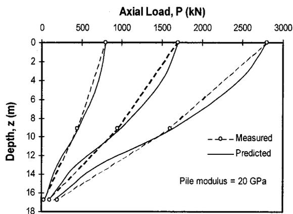
**Fig. 13.** Predicted and measured distributions of axial load along Piedmont pile
