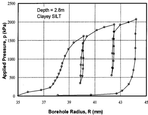
**Fig. 15.** Pressuremeter expansion curve at 2.8 m depth at Singapore test pile site
